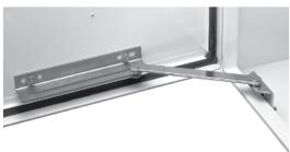
Designed for use with most standard, large mild and stainless steel enclosures to secure the door in the 90 degree open position. Door Stop Kit can be mounted at the top or bottom of the door opening after drilling two small holes in the door and enclosure. All parts are plated. Maintains UL/CSA Type 4 and Type 12 if properly installed in a Hoffman enclosure.
