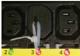
Cap secures in place with cable tie
