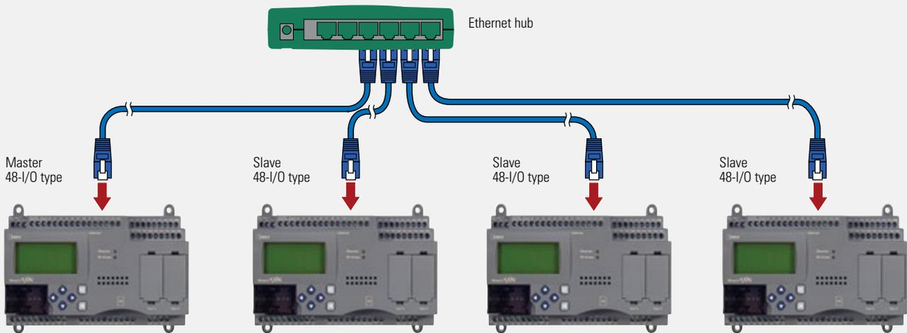
48-I/O type (master) + 48-I/O type (slave) + 48-I/O type (slave) + 48-I/O type (slave) = 192 I/O
