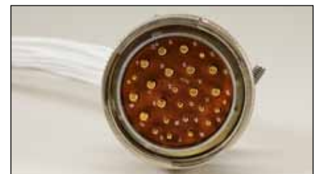
Connectors may contain several different size contacts.
