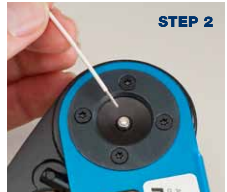
INSERT PRE-STRIPPED WIRE
