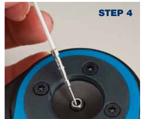
REMOVE TERMINATED WIRE ASSEMBLY
