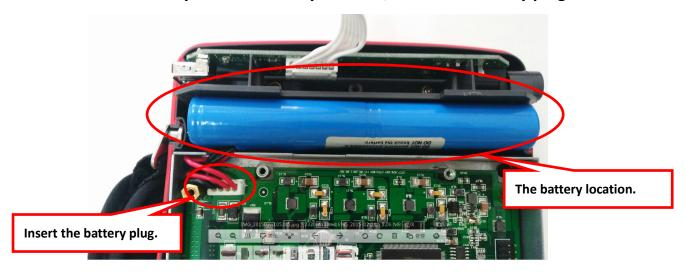
7. Reinstall the Fan plug, Power plug, Back cover and all screws.
