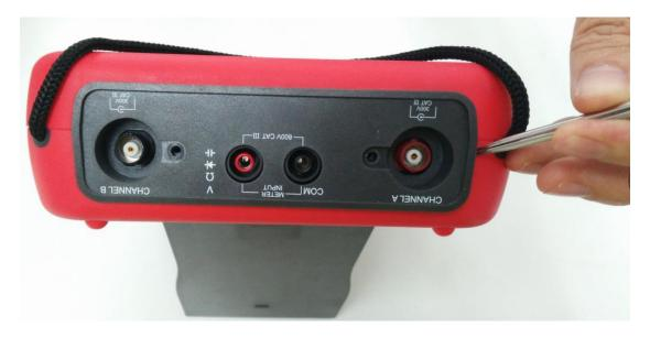
3. Remove the screw in red circle, then open the back cover.
