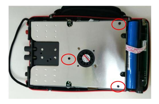
5. Remove the Fan cable and power cable , and open the cover.
