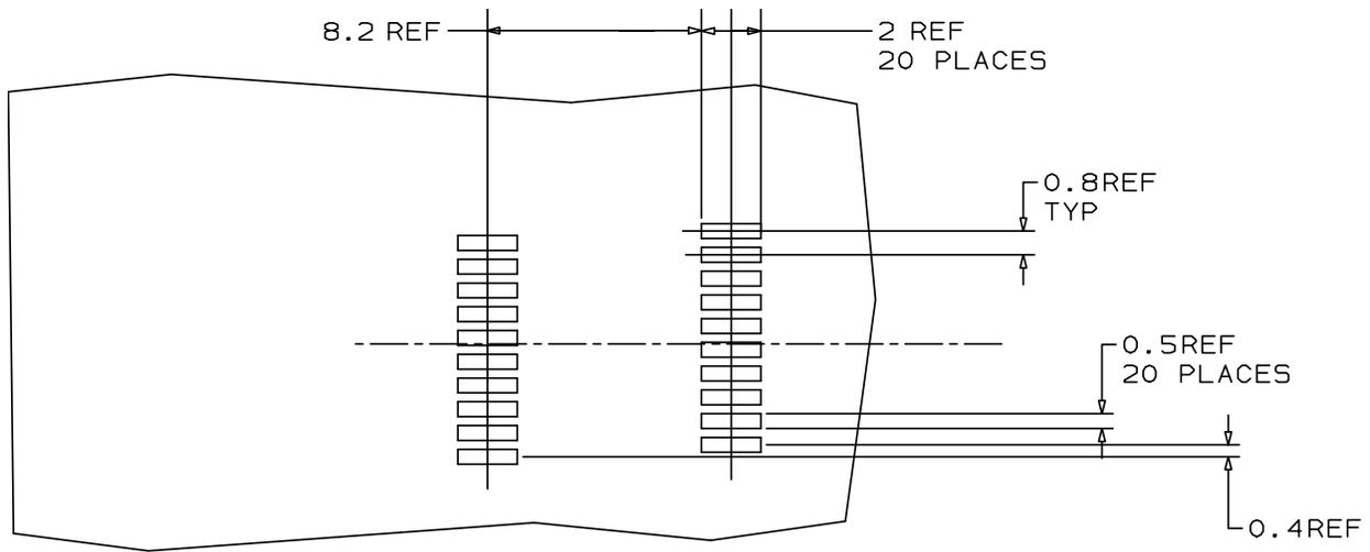
**NOTE:** For Specific Circuit Pad Locations, Refer to the Customer Drawing for the Specific Connector
