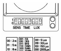
When power is connected, the load will turn on before the sensor times out and switches off. Once off, the load will switch back on when the sensor detects movement. If the sensor detects movement while the load is on, the on timer will be reset and the load stay on.
