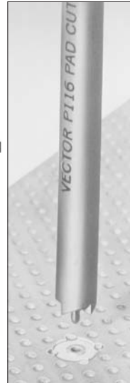
Shows pad removal & pad cutter P116C
