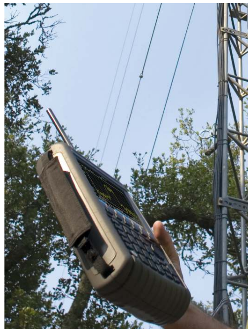
Use the spectrum analyzer's audio signal strength indicator to locate signals when walking around
