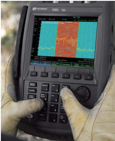
RF spectrum monitoring aided by spectrogram recording
