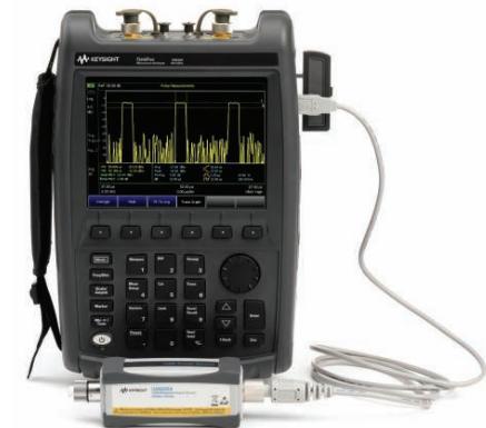
Keysight's FieldFox pulse measurements simplify radar field testing.
