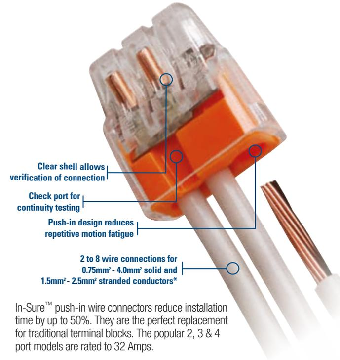
In-Sure™ push-in wire connectors reduce installation time by up to 50%. They are the perfect replacement for traditional terminal blocks. The popular 2, 3 & 4 port models are rated to 32 Amps.
