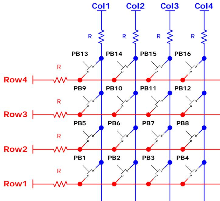
Figure 2-15. above shows the Symbolic representation of the Push Button Matrix KeyBoard. The following Figure 2-16. and Figure 2-17. shows the Symbolic representation of the Push button Switch Matrix KeyBoard with individual parts (Lower and Upper) Enabled using the Jumper setting. However, it is important to note that disabling a PB Matrix part physically isolates the PB Matrix part from the CPLD pins. When both the parts are enabled, the PB matrix becomes 4x4 Switch Matrix.
