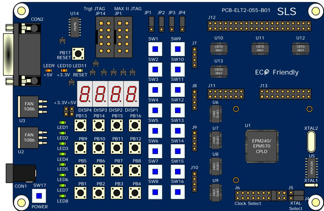
Figure 2-2. Below shows the Components on the Entry Level Tool - II Board.
