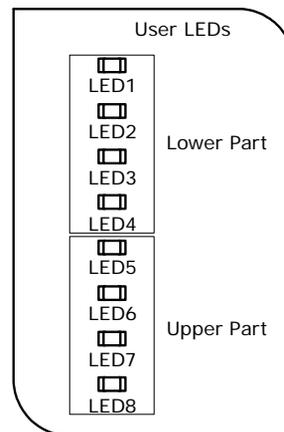
The LEDs on the ELT - II board are divided in two parts: Lower and Upper, each a group of 4 LEDs as shown in the figure above. Each part can be individually enabled or disabled by using a jumper selection option (**JP2** and **JP4**) as shown in the [Figure 2-13](#). below thus giving flexibility to the designer to use the LEDs as a group of 4 LEDs (Upper or Lower) or a group of 8 LEDs.
