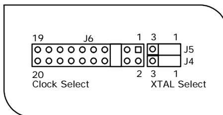
The clock circuitry of the Entry Level Tool - II board, basically, makes use of two crystals - 3.6864 MHz and 32.768 KHz. The crystal for the clock generator can be selected by making use of jumpers **J4** and **J5** as shown in the [Table 2-3](#) below:
