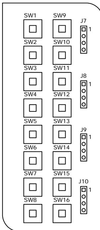
These 16 inputs are shared with IO headers (**J7** to **J10** as shown in the figure above), giving flexibility of additional 16 general purpose, +5V tolerant IOs to the designer. To use these headers as general purpose inputs/outputs, the designer must ensure that the switches are in IDLE (OFF) state to ensure that the Push Button Switch doesn't accidentally drive the shared IO line LOW (Logic "0").
