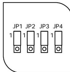
All the LEDs are connected in Common Anode configuration, and hence a logic LOW (Logic “0”) must be driven on the LED pin to turn ON the corresponding LED. The LED will turn on only if the respective LED part (Lower or Upper) is enabled. Disabling an LED part physically isolates the LED part from the CPLD pins. [Table 2-7](#) below gives the jumper selection option for enabling/disabling LED parts.
