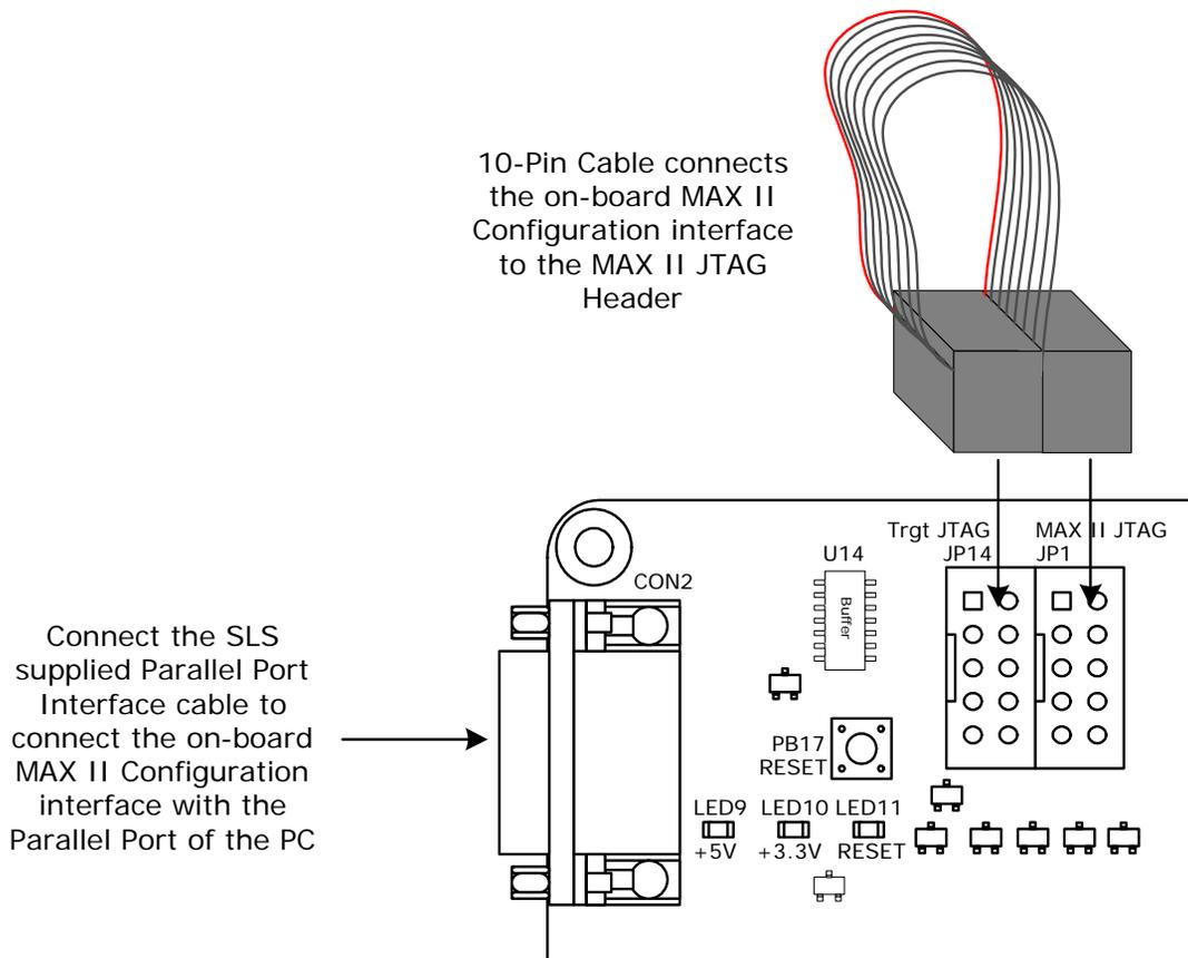
As shown in the figure above, connect the SLS supplied Parallel Port cable to the **CON2** connector on the Entry Level Tool - II Board, to get the PC connectivity. Use 10-Pin Cable supplied to connect **JP14** with the **JP1** to connect the on-board MAX II Configuration interface with the MAX II JTAG interface. Now the on-board device configuration interface is ready to be used with the Quartus II software to configure the MAX II device.
