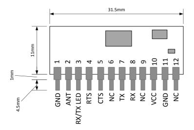
Pin Spacing: 2.54mm / 0.1" Pin Size: 0.6mm x 0.4mm
