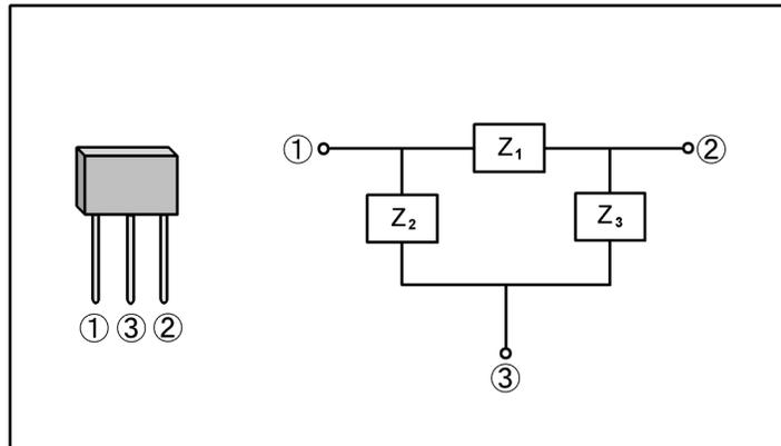
Use the guard terminal on the fixture to measure a 3-terminal device. Connect the lead No. 3 to the guard terminal in order to measure only characteristics of  $Z_1$  eliminating any effects from  $Z_2$  and  $Z_3$ .
