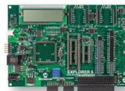
The Explorer 8 Development Kit is a full-featured development platform. It supports the largest number of 8-bit PIC microcontrollers ranging from 6 to 100 pins, making it the most versatile
