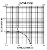
Gain using E51KF723 fibers, based on 90% reflective white card 2. 13150A Prism
