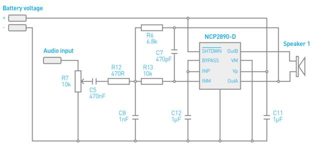
The audio amplification is performed by another Integrated Circuit or IC called an NCP2890-D. Inside the NCP2890-D are lots of transistors, which are connected together to allow the small input signal to be amplified into a more powerful output that can drive a speaker.
