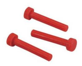
MS27488-8-3 connector grommet end sealing plugs from Aiconics can be used with connectors and terminal junction systems having wire sealing grommets conforming to: MIL-DTL-5015. These high quality connector sealing plugs can be installed in connector grommet cavity size 8.
