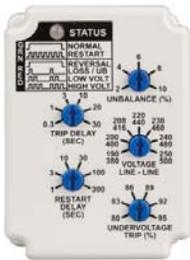
The Voltage Line-Line knob on the PMPU has two ranges (left): a 190-250V low voltage scale and a 380-500V high voltage scale. The unit auto senses the three-phase line-line voltage when applied and automatically selects the appropriate range.
