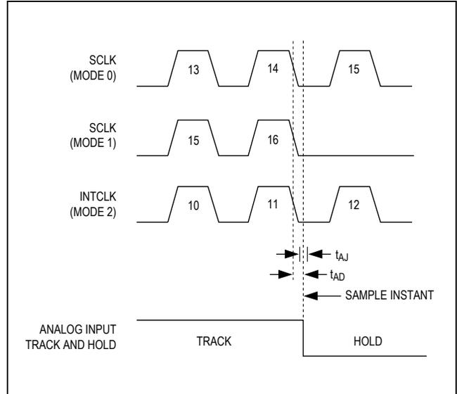
Figure 21. Aperture Diagram
