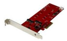
This M.2 SSD controller card lets you install two M.2 SATA solid-state drives (SSD) into your PC through PCI Express. You can mount virtually any M.2 drive directly to the card, giving you a convenient and discreet way to improve your computer system performance.
