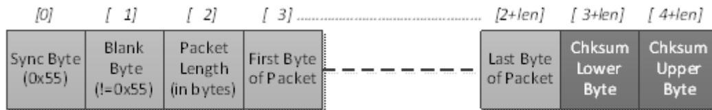
Serial Interface Packet with Transmission Rules Applied
