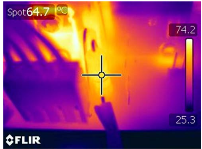
Figure 78 – Current Sense Resistor (R53), 230 VAC Input, 100% Load, Room Temperature.
