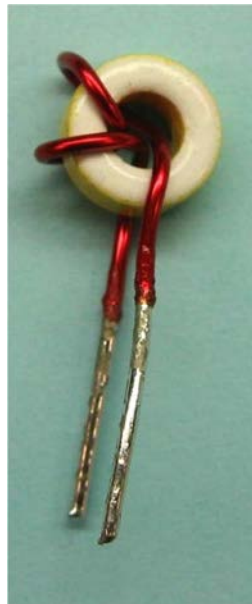
Figure 16 – Finished Part, Front View. Tin Leads to within ~ 1/8" of Toroid Body.
