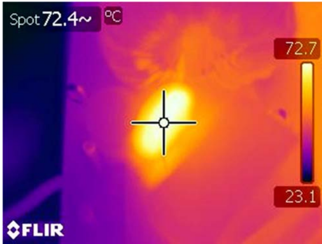
Figure 69 – Inrush Limiting Thermistor (RT1), 230 VAC Input, 100% Load, Room Temperature.
