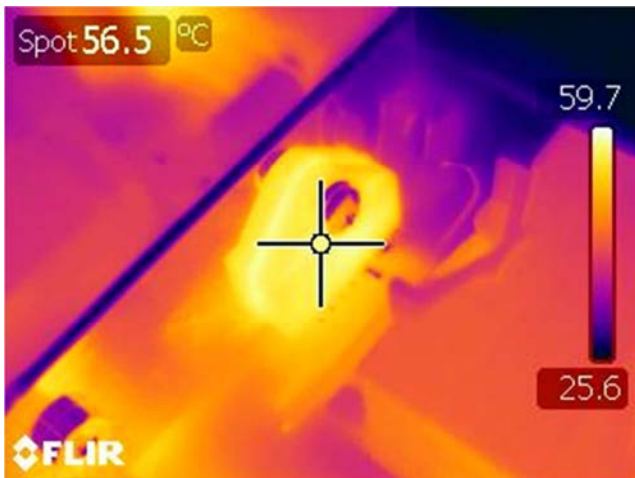
Figure 73 – PFC IC (U1), 230 VAC Input, 100% Load, Room Temperature.
