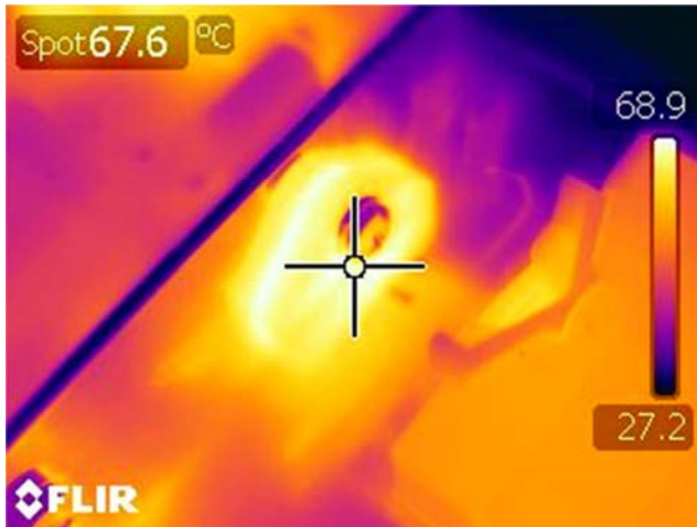
Figure 63 – PFC IC (U1), 115 VAC Input, 100% Load, Room Temperature.
