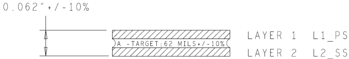
Figure 17. FRDM-CR20A PCB stackup cross-section (four layer)
