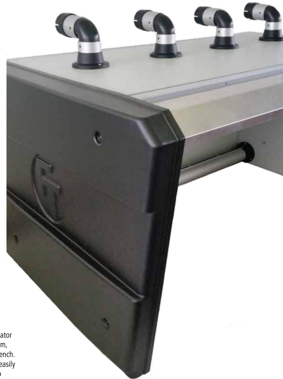
The air curtain cabinet CBC-A has a unique ventilation concept that separates the operator from the process by a dual air curtain system, giving unlimited accessibility on the workbench. It stands directly on the workbench and is easily connected to a FT mobile filter system or to central ventilation.
