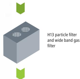
H13 particle filter and wide band gas filter
