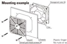
Plastic finger guards are placed on both the intake and exhaust sides of the fan. No nuts or screws for use in attachment included.
