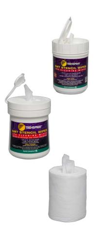
Lint-free, tear-resistant wipes saturated with 70% isopropyl alcohol and 30% deionized water (DI) for economical cleaning. The additional DI slows down dry time slightly, allowing more soak-in time for thicker and more difficult soils. Made of hydro-entangled polyester material. Ideal for surface cleaning, stencil and tool cleaning, and PCB cleaning.
