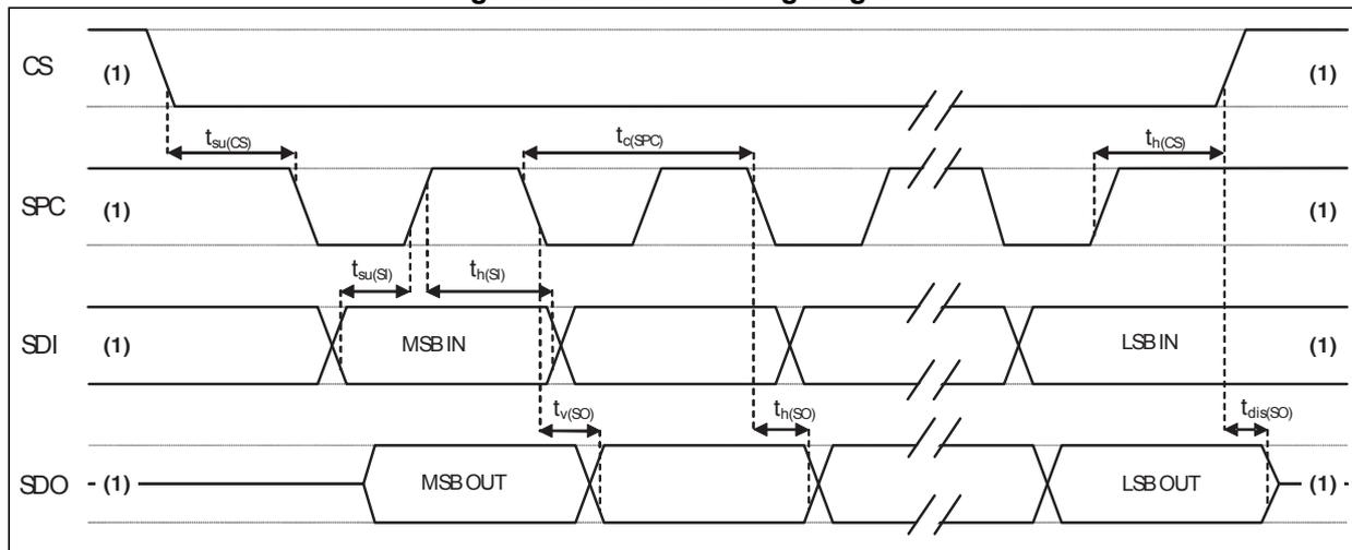
1. When no communication is ongoing, data on SDO is driven by internal pull-up resistors.
