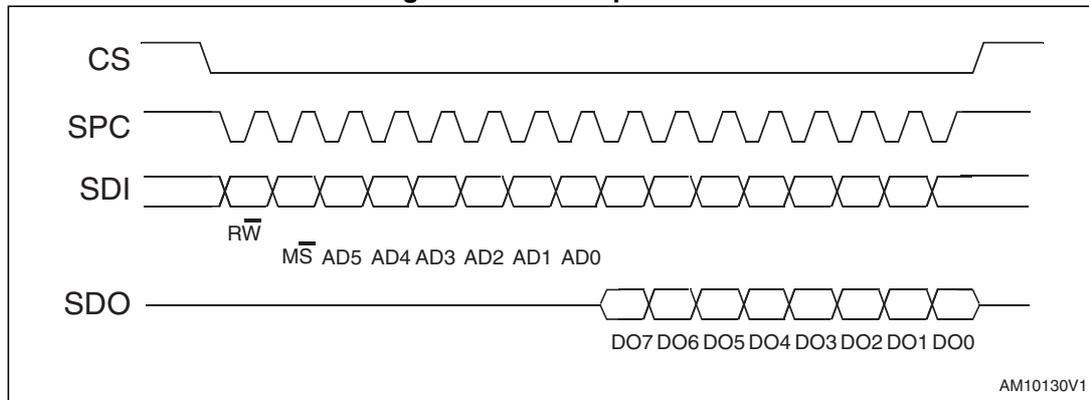
The SPI read command is performed with 16 clock pulses. A multiple byte read command is performed by adding blocks of 8 clock pulses to the previous one.
