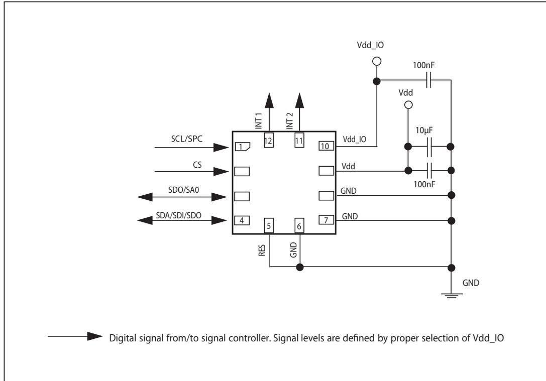
The device core is supplied through the Vdd line while the I/O pads are supplied through the Vdd\_IO line. Power supply decoupling capacitors (100 nF ceramic, 10 µF aluminum) should be placed as near as possible to pin 9 of the device (common design practice).
