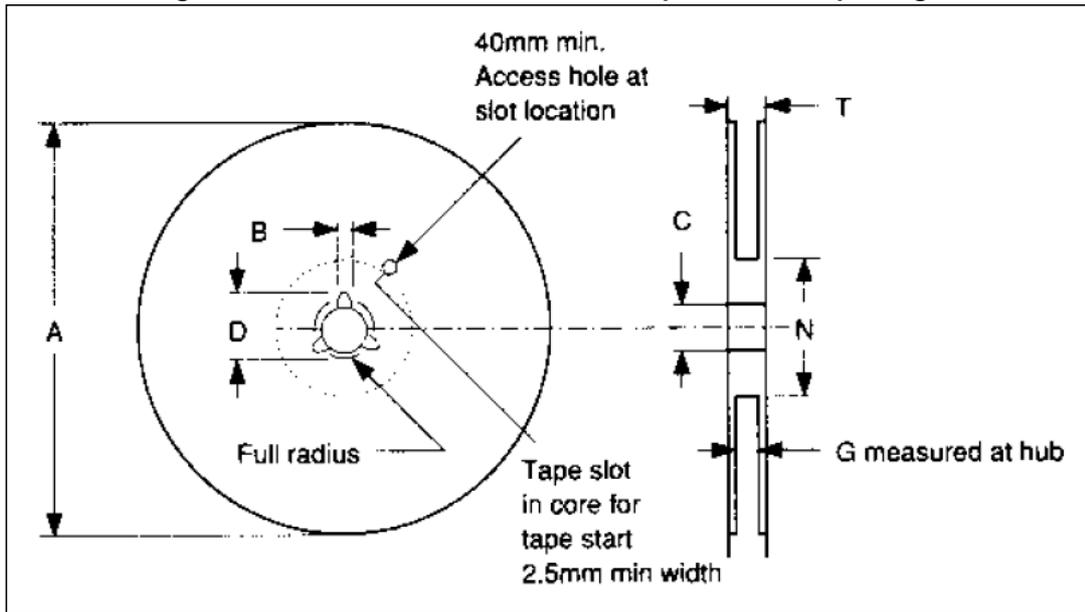
Table 83. Reel dimensions for carrier tape of LGA-12 package
