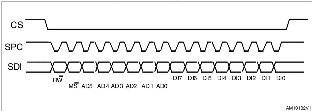
The SPI write command is performed with 16 clock pulses. A multiple byte write command is performed by adding blocks of 8 clock pulses to the previous one.
