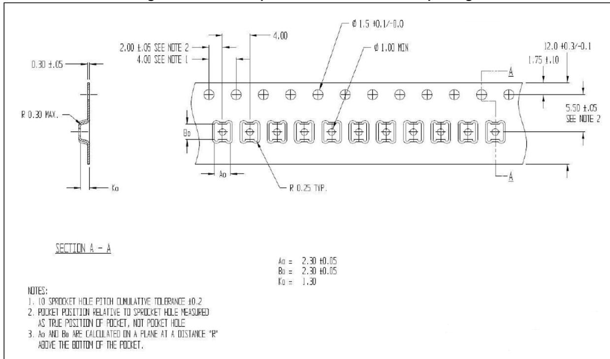
Figure 14. LGA-12 package orientation in carrier tape
