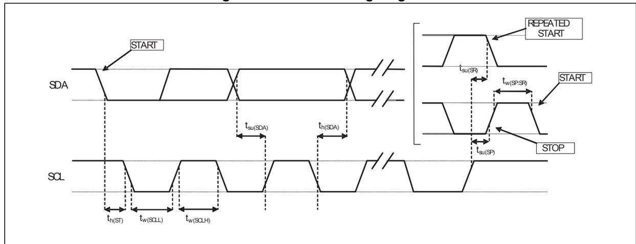
Note: Measurement points are done at 0.2·Vdd<sub>IO</sub> and 0.8·Vdd<sub>IO</sub>, for both ports.
