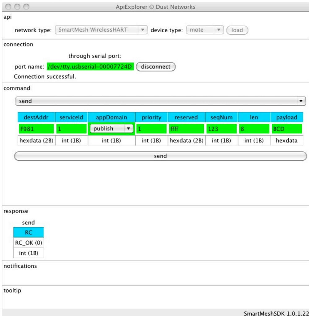
The screenshot shows the 'ApiExplorer' application interface. The 'network type' is set to 'SmartMesh WirelessHART' and the 'device type' is 'mote'. The connection is established through the serial port '/dev/tty.usbserial-00007724D'. The 'send' command is selected, and the following parameters are configured:
