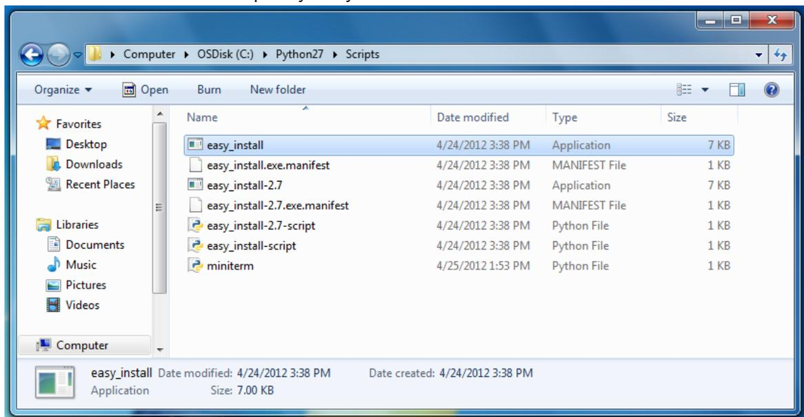
2. Install PySerial using the `easy_install.exe` script from the step above. The `easy_install.exe` script should be in your Python folder, e.g., `C:\Python27\Scripts`. (This folder might be a different place if you specified a different location when you installed Python.)
