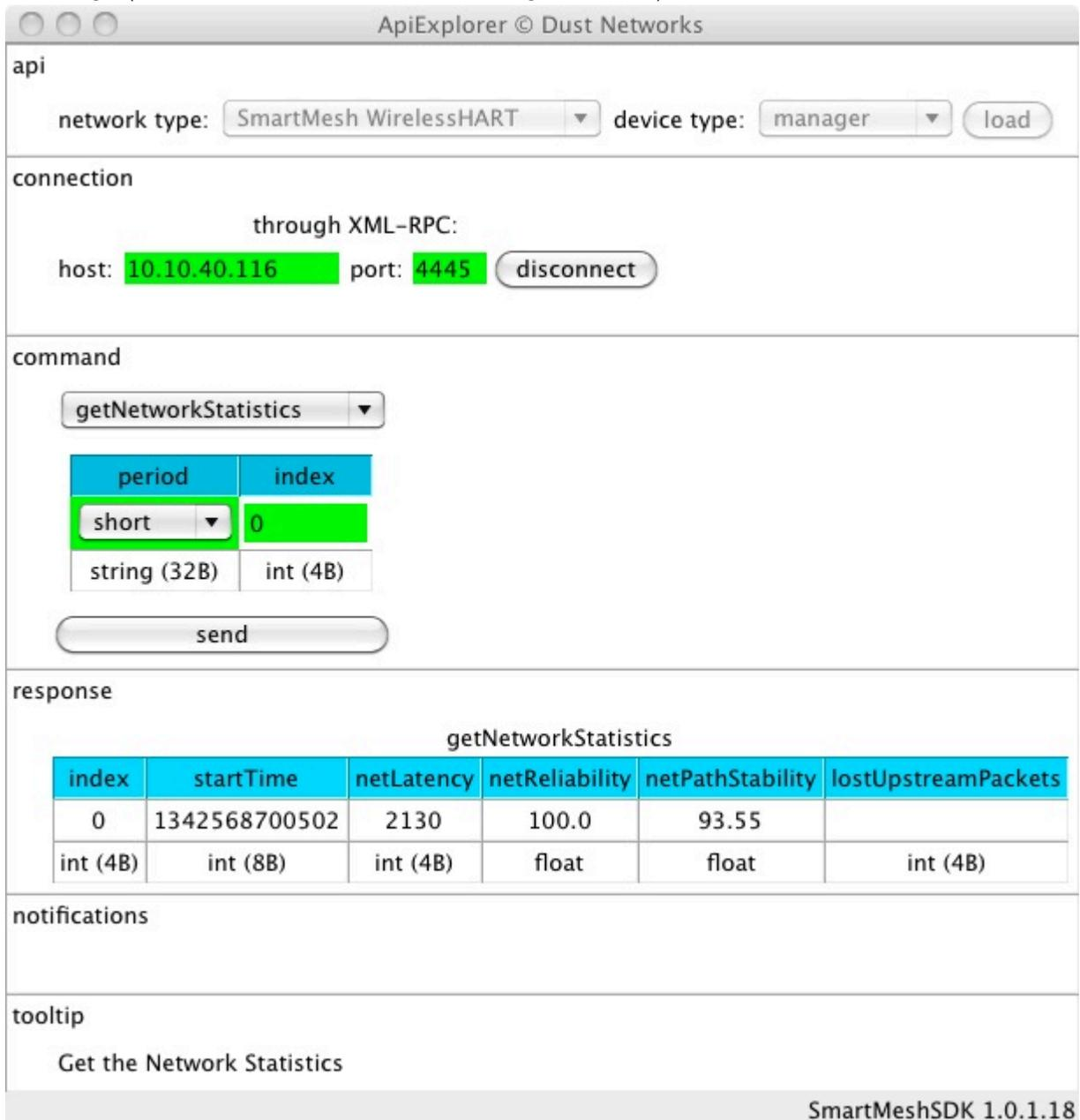
The screenshot shows the ApiExplorer interface for Dust Networks. It displays the configuration for the `getNetworkStatistics` command, including the network type (SmartMesh WirelessHART) and device type (manager). The connection details show the host as 10.10.40.116 and port as 4445. The command parameters are set to `short` for the period and `0` for the index. The response table shows the following data:
