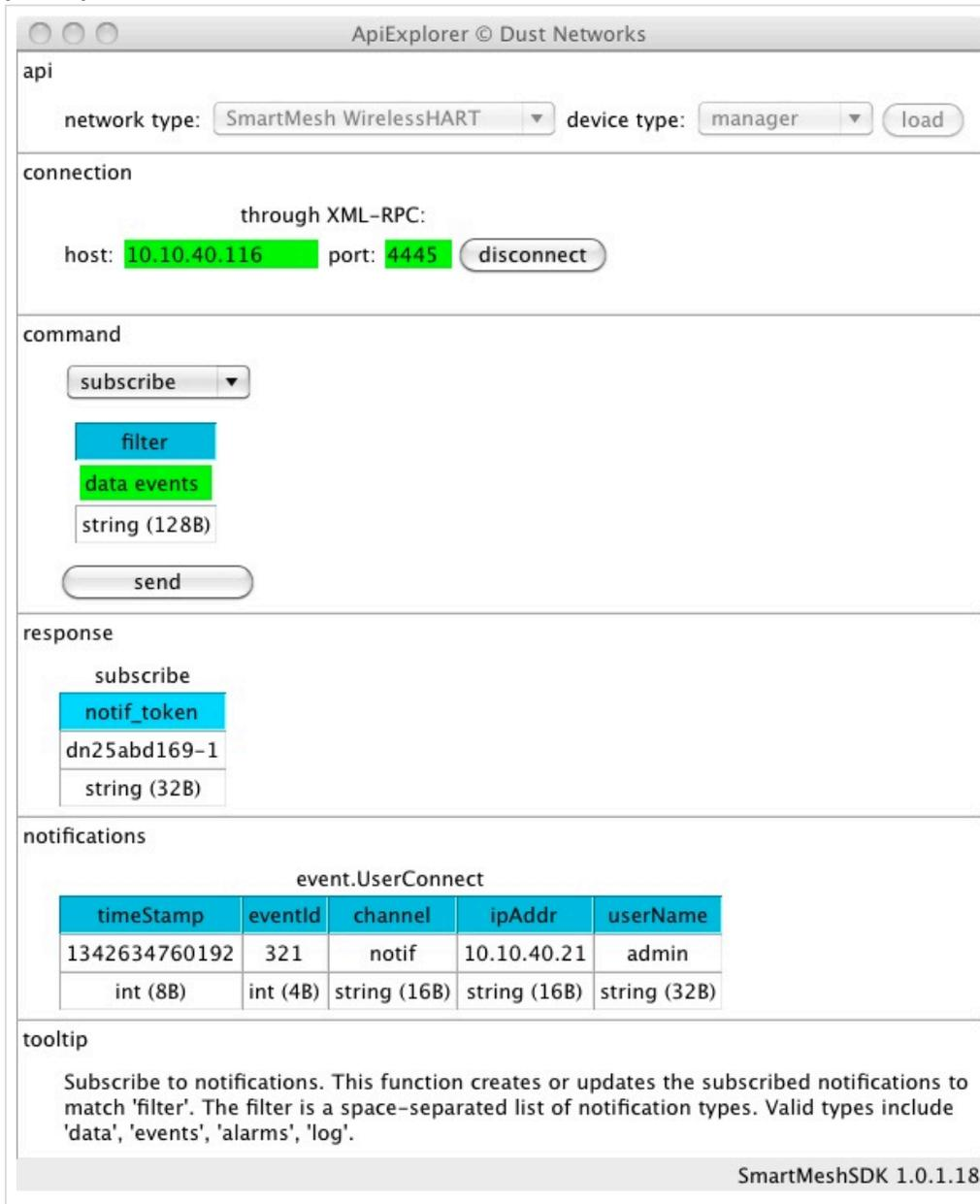
The screenshot shows the ApiExplorer interface for Dust Networks. It is configured for a SmartMesh WirelessHART network type and a manager device type. The connection is established through XML-RPC on host 10.10.40.116 and port 4445. The command 'subscribe' is executed with a filter of 'data events'. The response includes a 'notif\_token' of 'dn25abd169-1'. A notification table is shown below, indicating a successful connection event.
