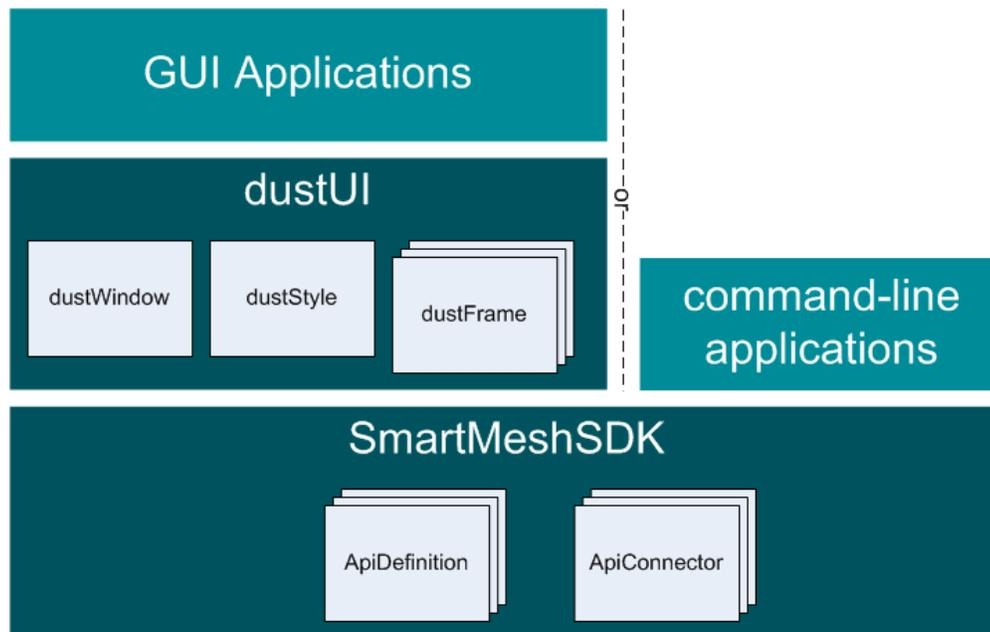
The SmartMesh SDK consists of three layers:
