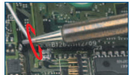
Rotate Tip Between Solder Joints
