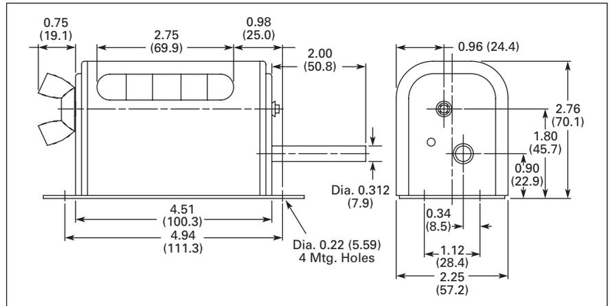
Figure 22. HDW Series — Approximate Dimensions in Inches (mm)
