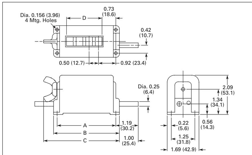
Figure 13. CS Series — Approximate Dimensions in Inches (mm)
