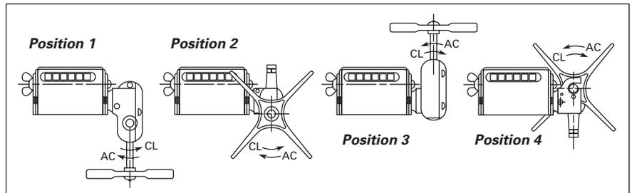
**Figure 31. HF Series — Can Counter Positions**
