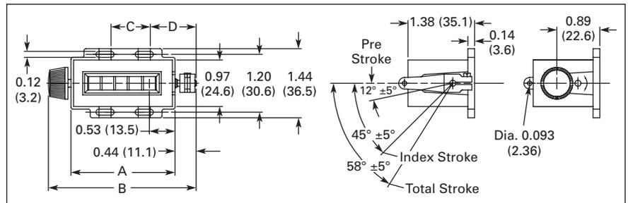
**Figure 1. X Series — Approximate Dimensions in Inches (mm)**
