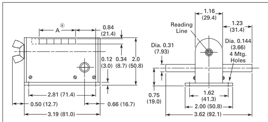
Figure 19. D-6 Series — Approximate Dimensions in Inches (mm)
