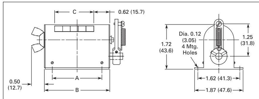
Figure 5. D Series — Approximate Dimensions in Inches (mm)
