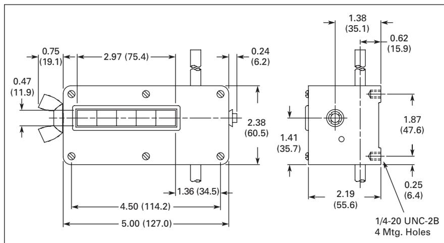
Figure 25. T Series — Approximate Dimensions in Inches (mm)
