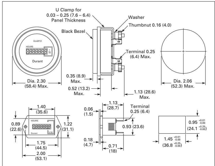
**Figure 57. E42DI24/E42DIR Series — Approximate Dimensions in Inches (mm)**
