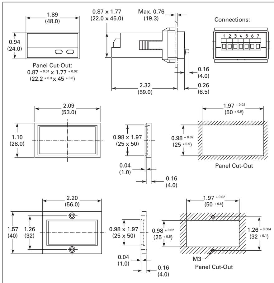
Figure 54. E5-324-E Series — Approximate Dimensions in Inches (mm)
