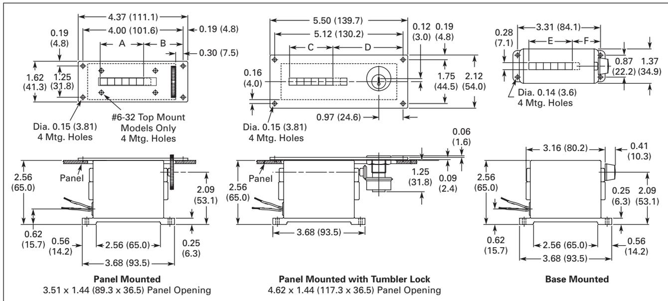
Figure 35. MF Series — Approximate Dimensions in Inches (mm)
