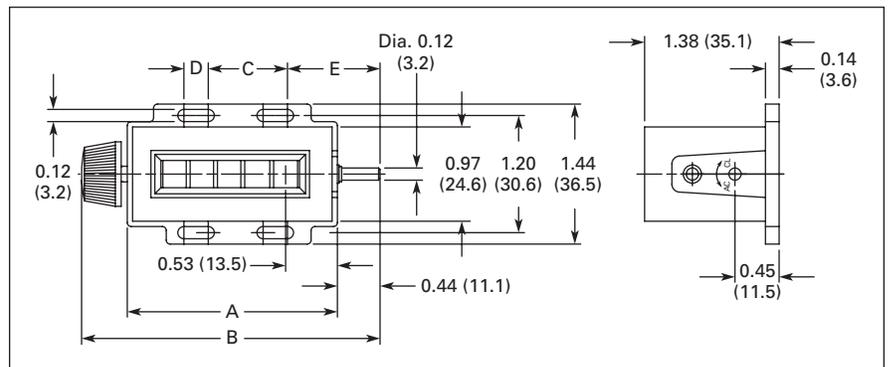
Figure 8. X Series — Approximate Dimensions in Inches (mm)
