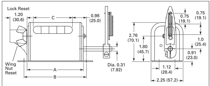
**Figure 4. H Series — Approximate Dimensions in Inches (mm)**
