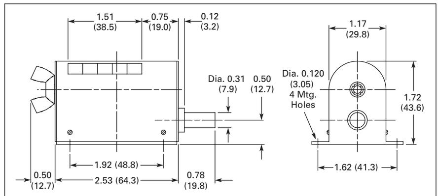
Figure 16. D-7 Series — Approximate Dimensions in Inches (mm)
