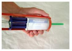
Remove the cap from the cartridge and affix a static mixing nozzle.
