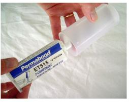
Slot the 50ml cartridge into the oval end of the translucent cylinder.
