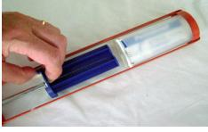
The blue plunger fits onto the gun's plunger. Squeeze the trigger, aligning the plungers with the back pistons on the cartridge.
