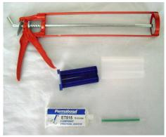
1 You will require a 320ml mastic gun into which the converter will fit
