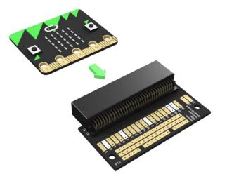
**Examples of board in use:** This breakout board is used in our 'Inventors kit for BBC micro:bit'. This kit is supplied with instructions detailing a number of uses for the board. These can be found at <u>www.kitronik.co.uk/microbitinvent</u>
