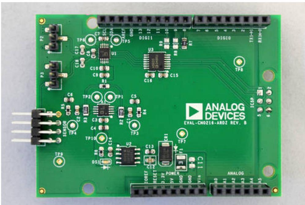
This circuit allows great flexibility in designing a custom low-level signal conditioning front end that gives the user the ability to easily optimize the overall transfer function of the combined sensor-amplifier-converter circuit. The [AD7791](#) maintains good performance over the complete output data range, from 9.5 Hz to 120 Hz, which allows it to be used in weigh scale applications that operate at various low speeds.
