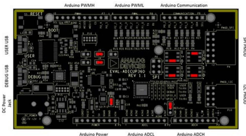
The `ADuCM360_cn0326_demo` uses **UART** connection via **P0.6/P0.7** and **SPI0** channel of the ADuCM360 to communicate with CN0326 board.
