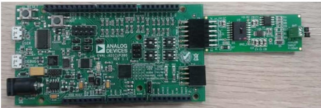
The CN0336 circuit consists of an input current-to-voltage converter, a level shifting circuit, an ADC stage and an output isolation stage. The **4 mA to 20 mA** input signal is converted into **voltage** levels compatible with the input range of the ADC (**0 V - 2.5 V**). The 12-bits ADC value is received via SPI interface of the EVAL-ADICUP360 board.
