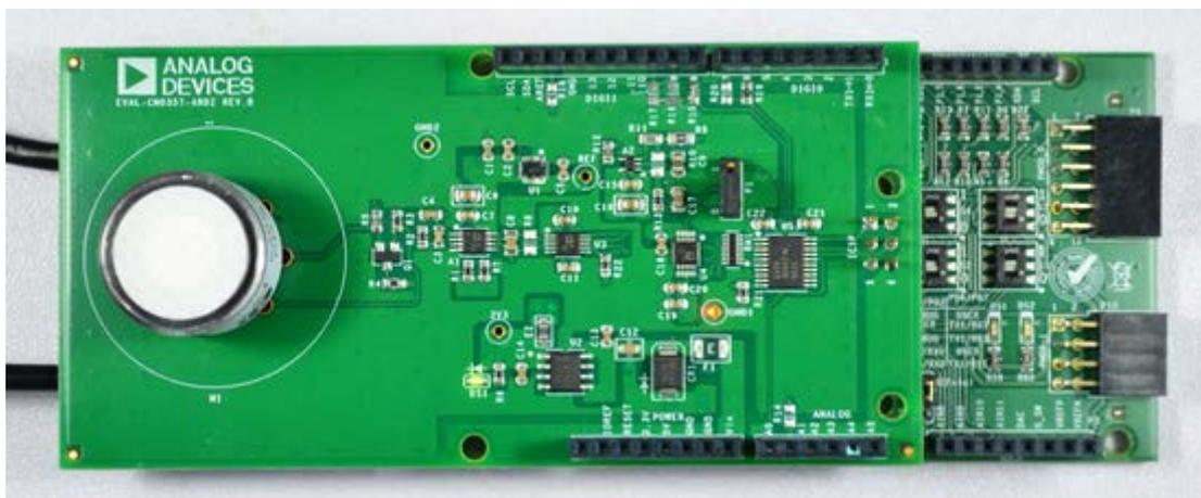
The [EVAL-CN0357-ARDZ shield](#) circuit provides a potentiostatic circuit for biasing the electrochemical sensor, along with a programmable TIA and 16-bit Sigma-Delta ADC. The TIA converts the small currents passing in the sensor to a voltage that can be read by the ADC. The 16-bit ADC value is received via SPI interface of the EVAL-ADICUP360 board, where the gas concentration is computed.
