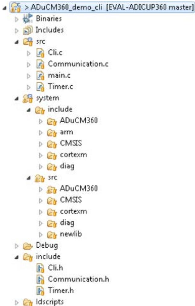
This project contains: initialization part - disabling watchdog, setting system clock, enabling clock for peripheral; UART interrupt service; port configuration for UART use; UART read/write management; command line interpreter application.
