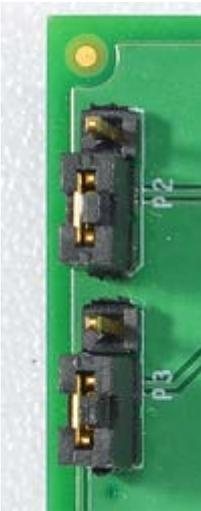
Position "1" is used for 4-wire resistive bridges
