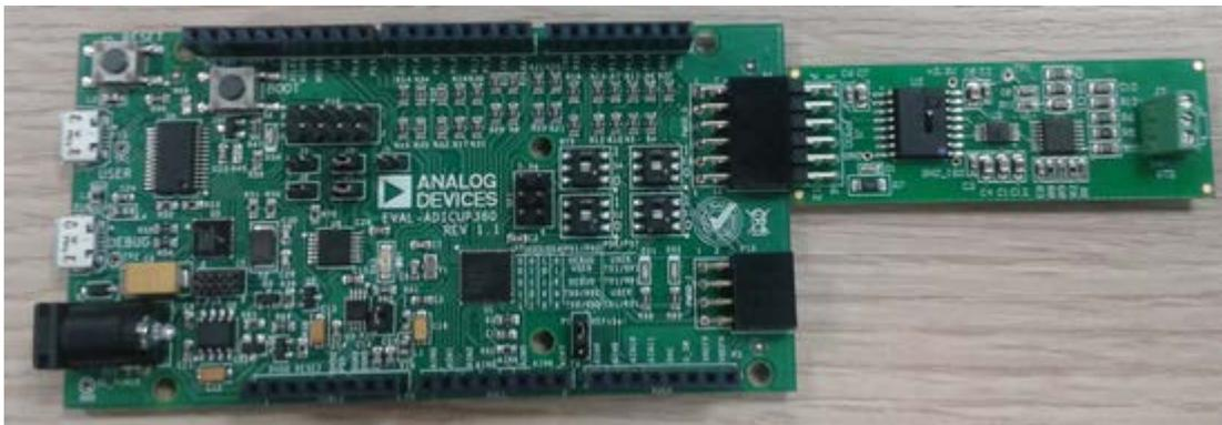
The CN0337 circuit translates the **RTD** input **resistance** range (**100  $\Omega$  - 212.05  $\Omega$**  for a **0°C - 300°C**
