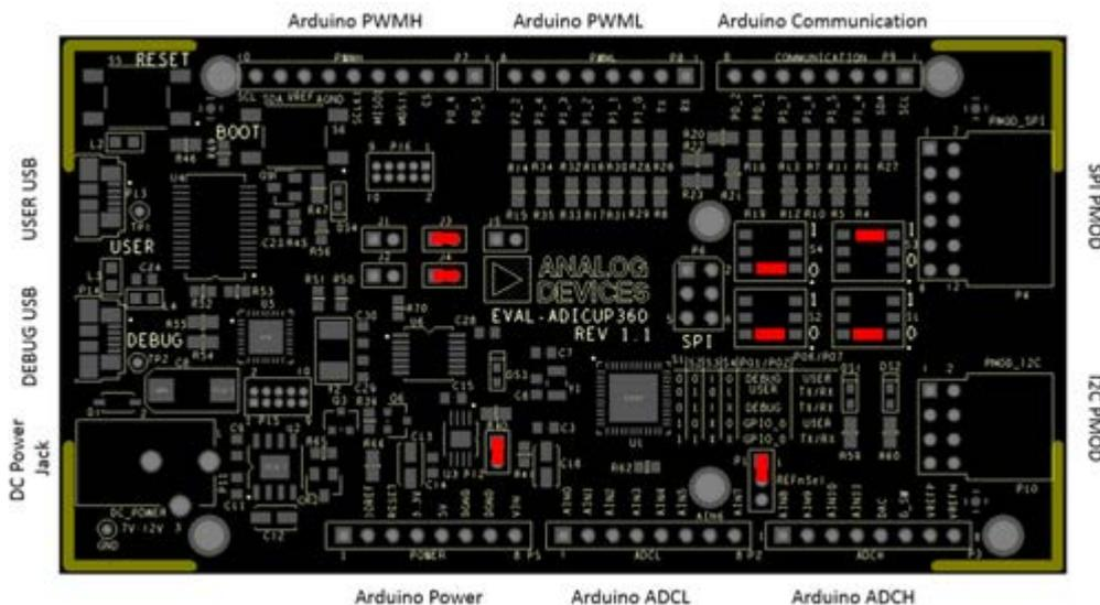
The ADuCM360\_cn0336\_demo use **UART** connection via **P0.6/P0.7** and **SPI0** channel of the ADuCM360 to communicate with CN0336 board.
