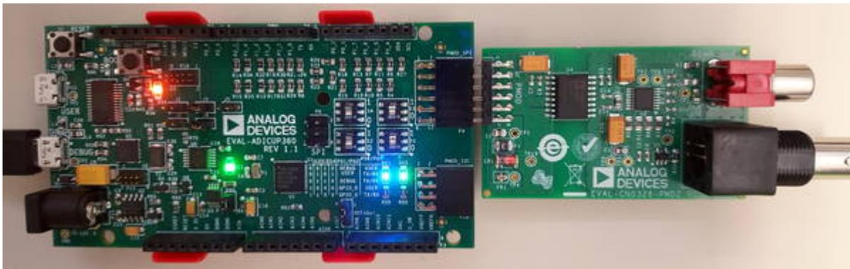
The CN0326 circuit provides a complete solution for pH sensors with internal resistance between **1 M $\Omega$**  and several **G $\Omega$** . It consists of **pH probe** buffer, **Pt1000 RTD** for temperature compensation and **24-bits ADC** with 3 differential analog inputs.
