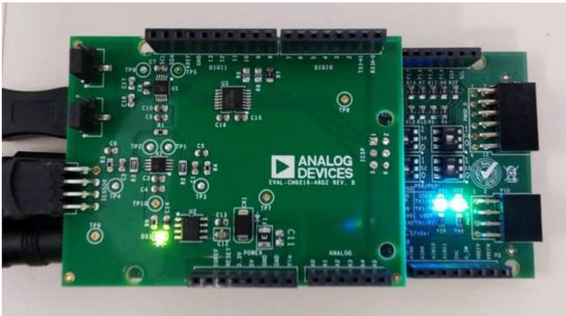
The CN0216 circuit translates the resistance changes on the bridge into very small voltages. The bridge is excited by a regulated 5V and that determines the full scale range of the bridge output. Those
