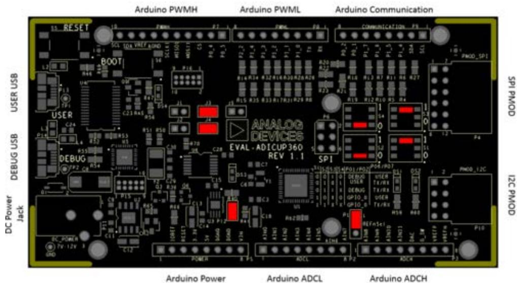
The ADuCM360\_demo\_cn0216 uses **UART** connection via **P0.6/P0.7** and **SPI1** channel of the ADuCM360 to communicate with [EVAL-CN0216-ARDZ shield](#).
