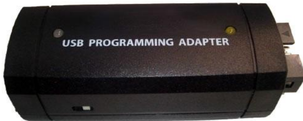
Figure 3. Novato USB-to-UART programming adapter.
