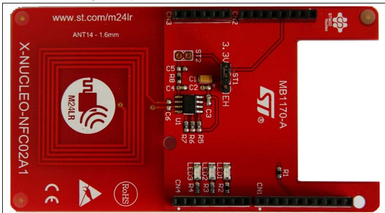
Figure 1. Expansion board based on M24LR04E-R for STM32 Nucleo
