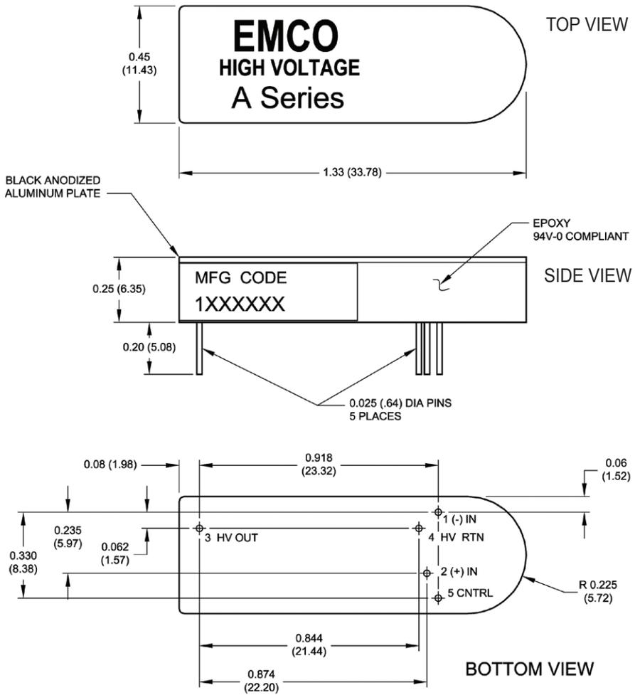
DIMENSIONS ARE IN INCHES (METRIC EQUIVALENTS ARE IN PARENTHESIS)
