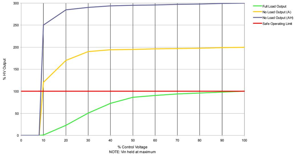
Typical Input vs. Output Voltage
