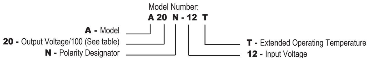
EXAMPLE: **A20N-12T** (**A** - Model, **20** - Output Voltage, **N** - Negative, **12** - Input Voltage, **T** - Extended Operating Temperature)
