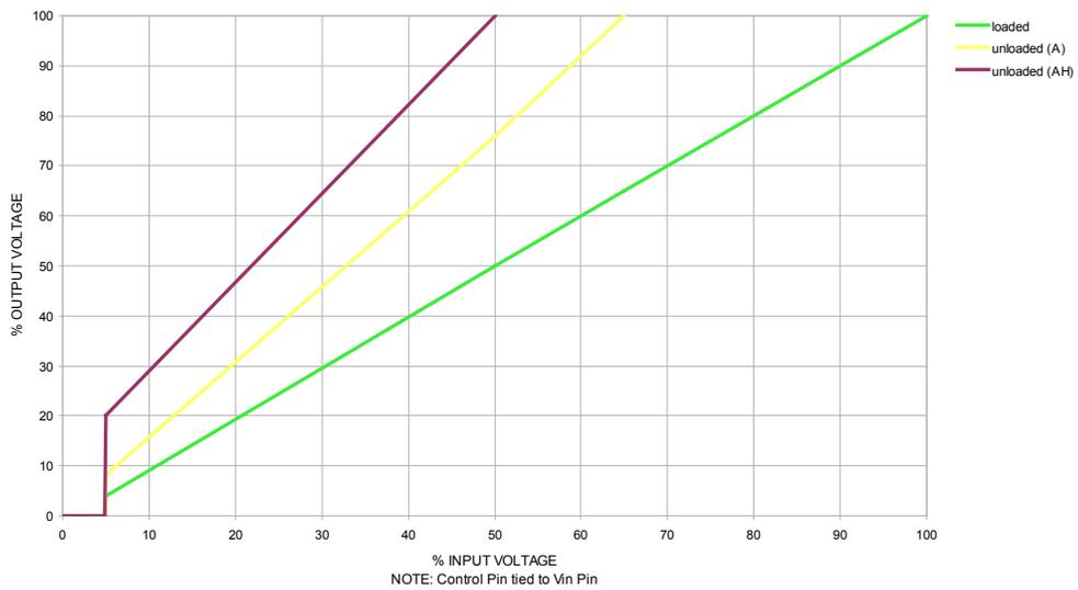
Output Voltage is load dependent. Under light or no-load conditions, reduce the Input Voltage so maximum rated Output Voltage is not exceeded.
