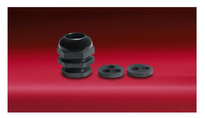
A Moulded Cable Gland Kit for Wylex NM Metal Consumer Units providing additional support and supplementary insulation similar to Class II construction for the incoming cables. Suitable for a 32mm round entry point and meter tails of 25mm² plus 16mm² earth conductor and meter tails of 16mm² plus 10mm² earth conductor.
