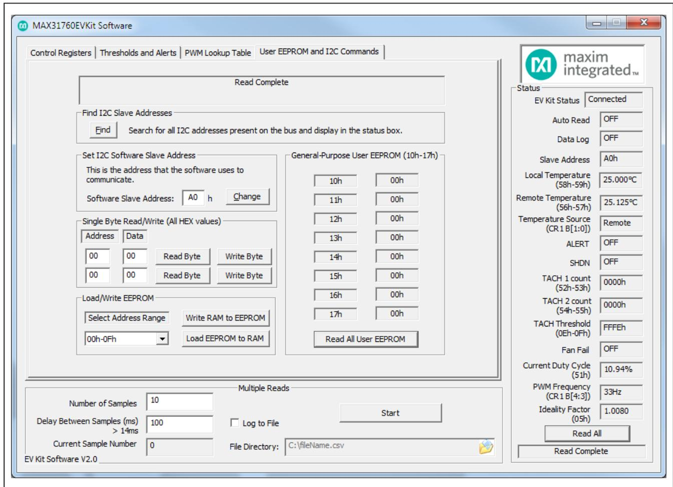
Figure 4. MAX31760 EV Kit Software (User EEPROM and I<sup>2</sup>C CommandsTab)
