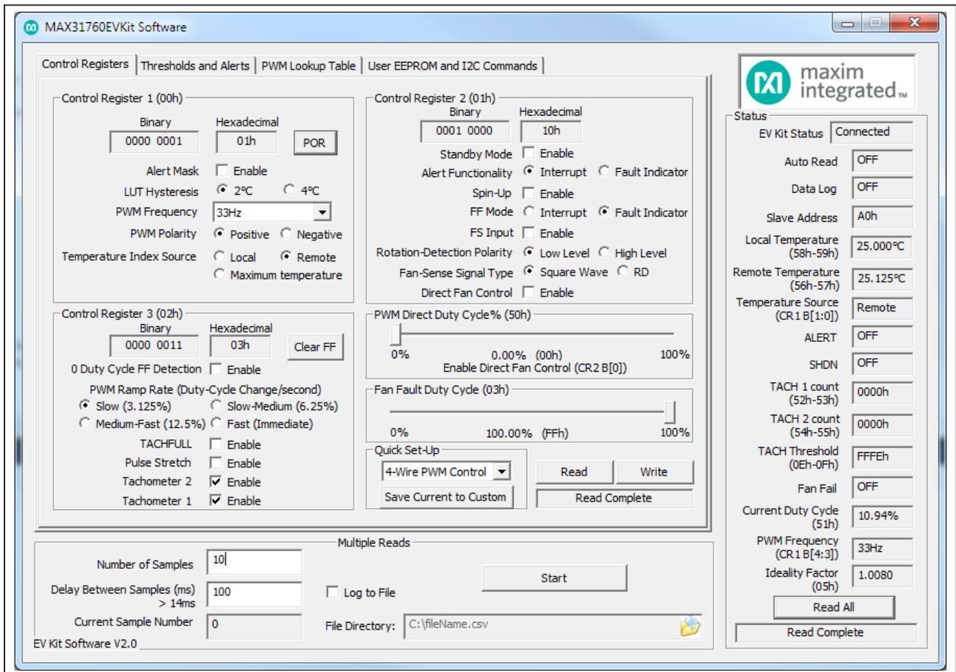
Figure 1. MAX31760 EV Kit Software (Control Registers Tab)
