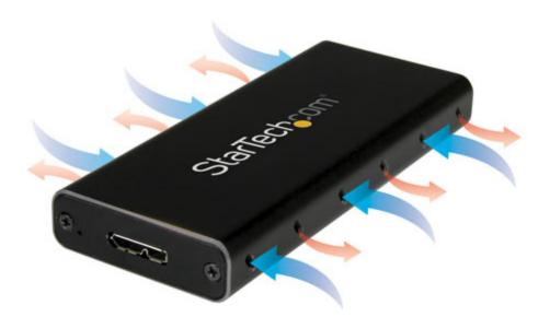
The mSATA enclosure provides dependable drive protection with its durable, solid aluminum housing. It also features ventilation holes to help protect your drive from overheating by allowing heat to dissipate and
