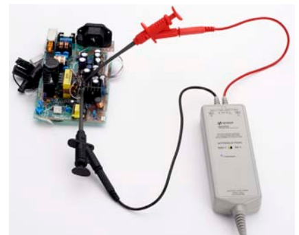
N2790A measuring a power supply signal
