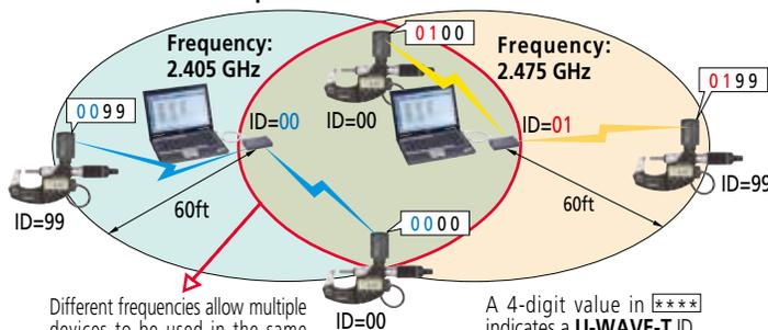
Different frequencies allow multiple devices to be used in the same communication range.
