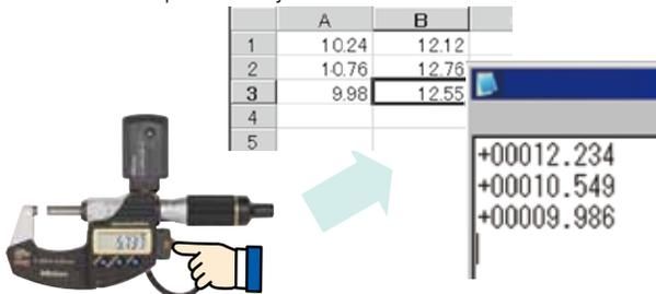
In addition, a virtual COM driver allows measurement data to be input to a program that supports **RS-232C** serial communication. The communication speed (baud rate) is fixed to 57,600 bps.
