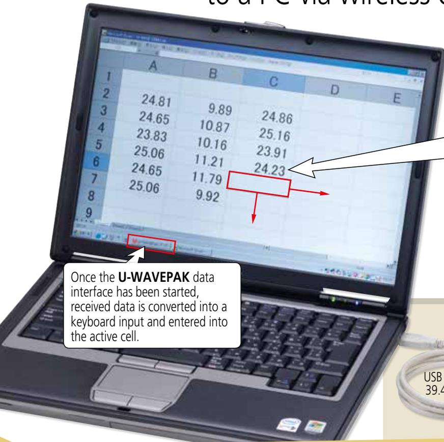
When the data input button is pressed, the value displayed on the measuring tool is entered into the active cell of Excel followed by "Enter" key input. The cursor movement direction after input (up, down, left or right) can be set in Excel.
