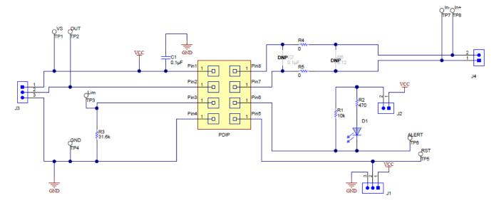
Figure 2. INA301EVM Test Board Schematic
