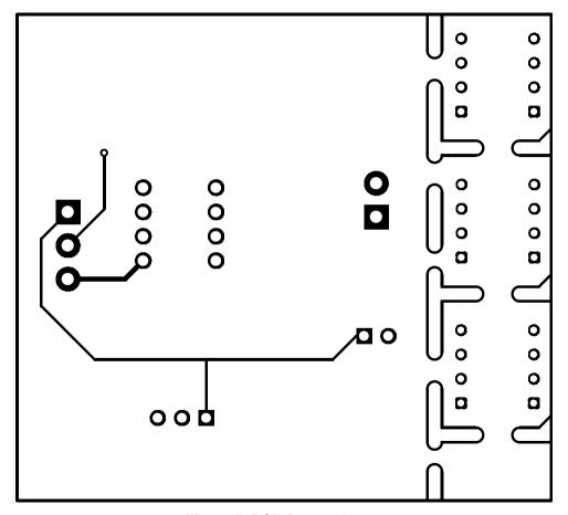
Figure 5. PCB Bottom Layer
