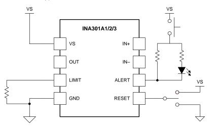
Figure 1. INA301EVM Test Board Block Diagram
