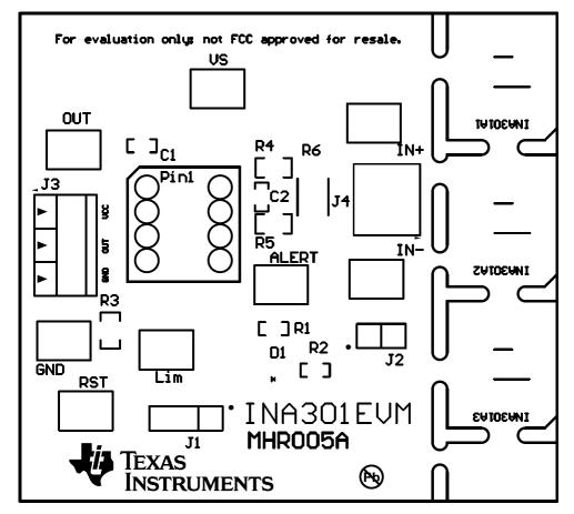
Figure 3. INA301EVM Component Placement
