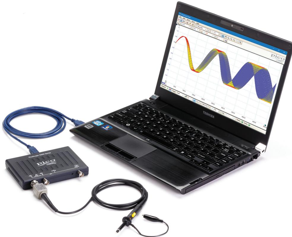
The PicoScope 2000 Series' use of hardware acceleration means that, in Fast Persistence mode, waveform update rates of up to 80 000 waveforms per second can be achieved (model-dependent), overlaying them all with color-coding or intensity-grading to show which areas are stable and which are intermittent. Faults that previously took minutes to find now appear within seconds.
