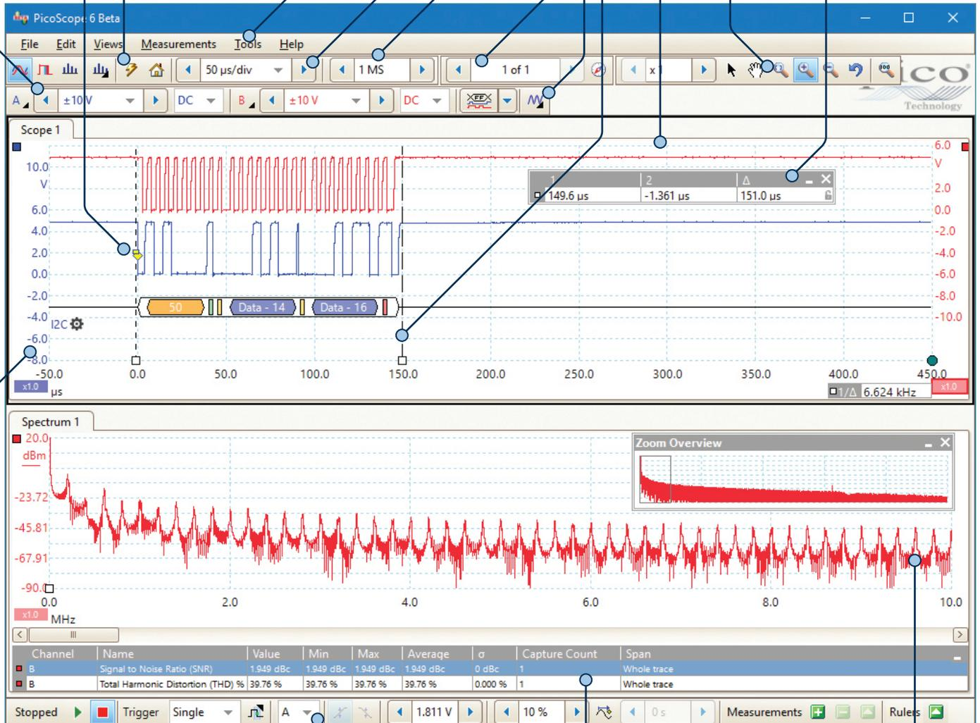
**Movable axes:** The vertical axes can be dragged up and down. This feature is particularly useful when one waveform is obscuring another. There's also an Auto Arrange Axes command.
