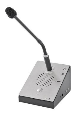
The DTS1 is a vandal resistant, desktop intercom station consisting of a 30C25Z80T - 3'' square frame loudspeaker with a 2.35oz. ceramic magnet and a moisture resistant cone, a push-to-talk (PTT) button and a removable 18'' gooseneck microphone. Stainless steel faceplate with 3 interwoven, steel security screens mounted between the loudspeaker. Console finish is black powder coat.
