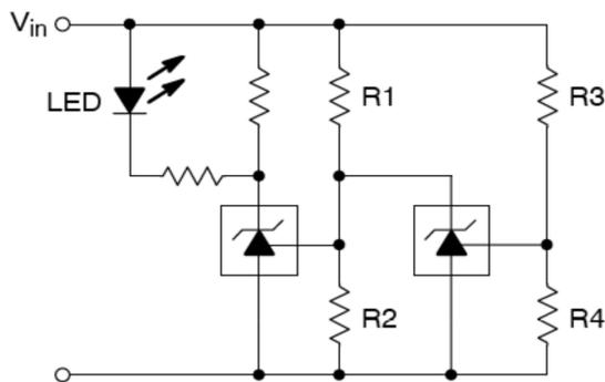
L.E.D. indicator is 'ON' when  $V_{in}$  is between the upper and lower limits,
