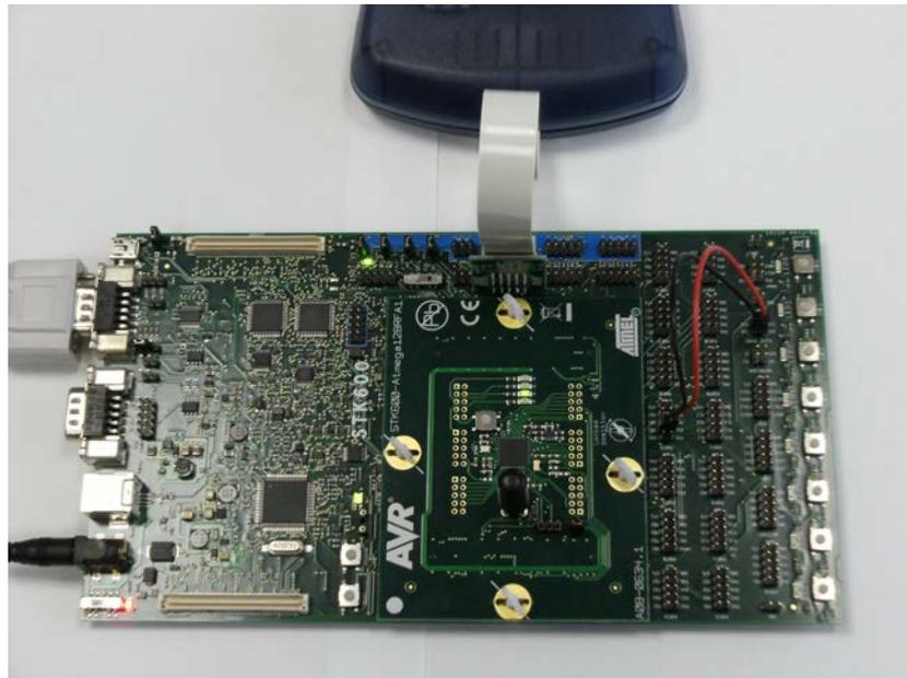
**Figure 10-25.** Atmel ATmega128RFA1-EK1 wiring for UART1.
