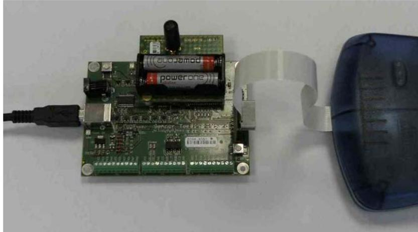
The Sensor Terminal Board can be powered with USB, although it is recommended to use a powered hub in case the board is not directly connected to a PC.
