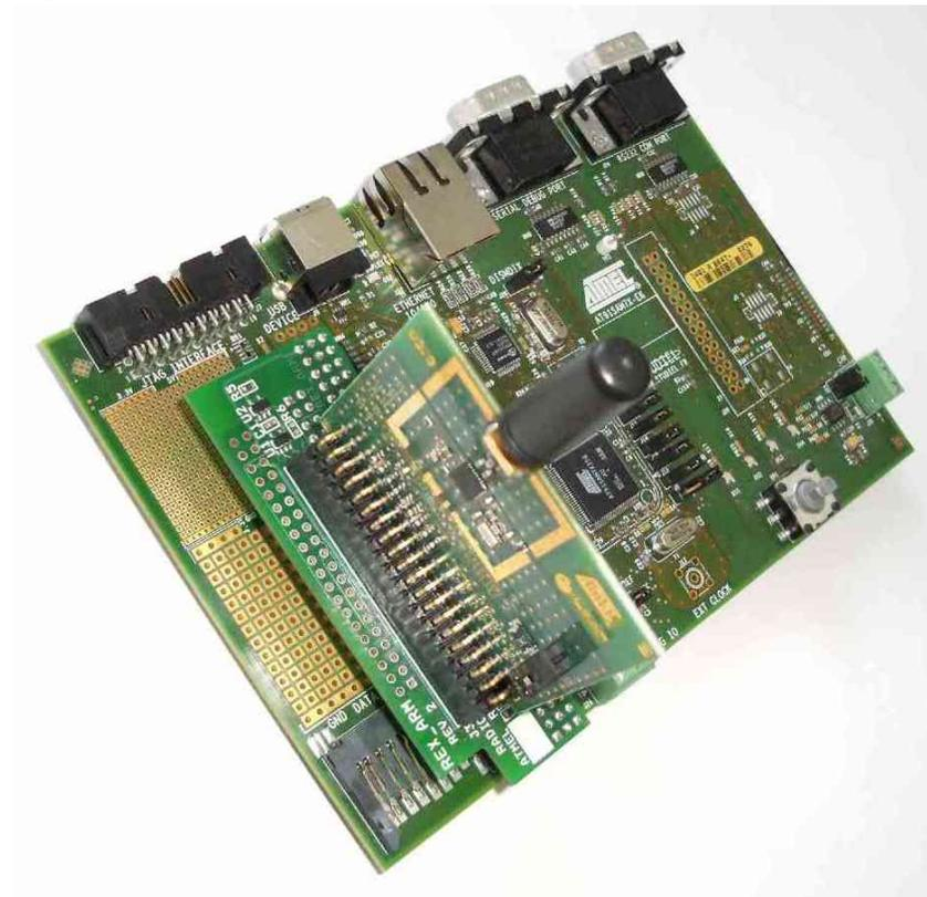
**Figure 10-22.** Atmel AT91SAM7X-EK board with Atmel AT91SAM7X256 connected to Atmel SAM-ICE and UART.
