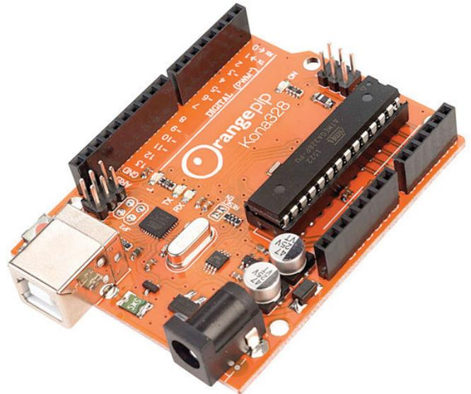
microcontroller and other components on the board. This can come either from VIN via an on-board regulator, or be supplied by USB or another regulated 5V supply.
