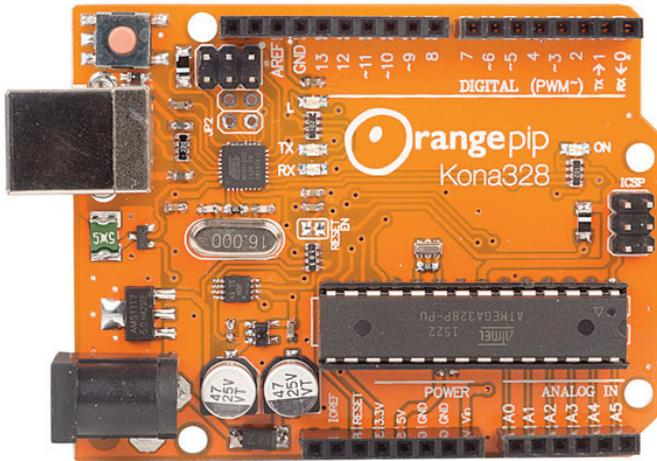
**LED: 13** There is a built-in LED connected to digital pin 13. When the pin is HIGH value, the LED is on, when the pin is LOW, it's off.
