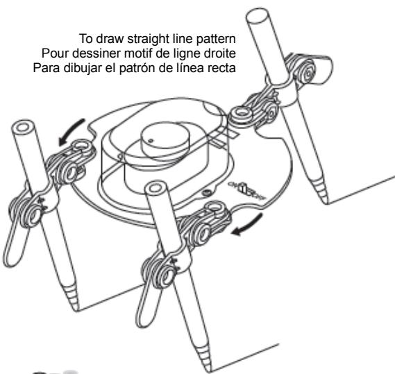
4. When the vibration brush mounted on the robot, the robot will dance around. Adjust the direction and angle of vibration .
