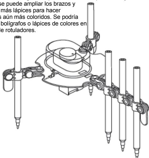
**6.** Remove all the pens and turn down the arm ends . Doodling robot becomes a vibrobot that slides across smooth surfaces .
