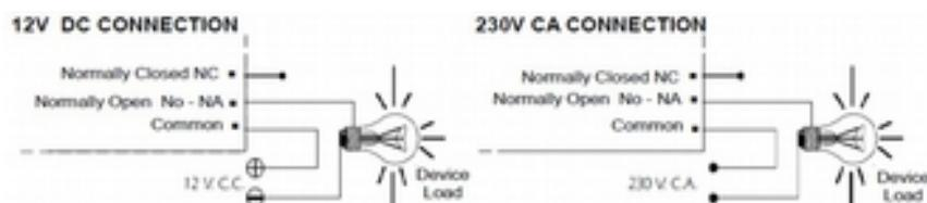
**INFORMATION ABOUT THE OUTPUT.** During the operating mode and according to its load, it could happen a fluctuation or an incorrect working of the output. In such case, you have to install an anti-spark circuit (100 nF/400V Capacitor type X2 and 47 . ½ W resistor) between both contacts of the used relay, as it is indicated on the drawing.
