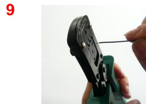
9 Insert the cable until insulation Stop blade.
