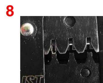
8 Close the tool lightly until the contact is held (1. Ratchet Lever).
